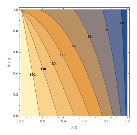
Contour plot of the scattering angle (in degrees) of the light puck as a function of the fractional impact parameter and the mass ratio. The scattering is exactly backward ( $\theta$ = 180°) along the left edge of the graph for an on-center collision (b = 0) and is exactly forward ( $\theta$ = 0°) along the right edge of the plot for a grazing collision (b = D).
