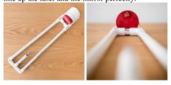
Once the laser is hitting the center of the plastic mirror, check to make sure that a crisply reflected laser spot is visible.
