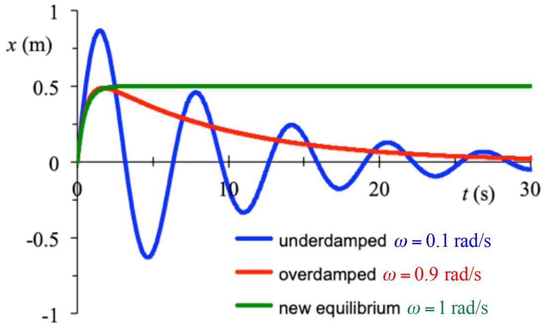
Parameters:  $m = 1$  kg,  $2\kappa = 1$  N/m,  $\mu = 1$ , and  $\dot{x}_0 = 1$  m/s  $\Rightarrow \omega_c^* = 0.71$  rad/s and  $\omega_c = 1$  rad/s.
