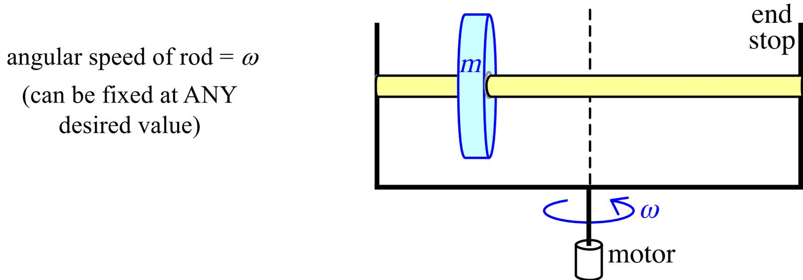
The end stops prevent the bead from sliding off the rod.
